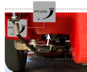
The water quantity can be adjusted for any floor covering.
