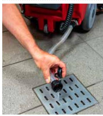
The clean water tank can be fully drained.
