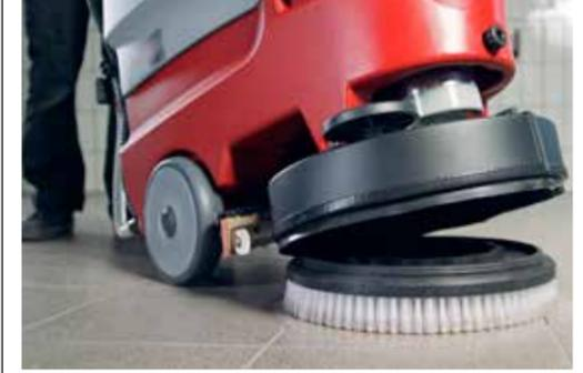
Comfortable brush ejection at the push of a button.
