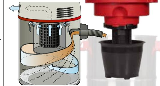
Due to the twist of the intake nozzle, the spray-fog is consequently diverted along the inner container wall. Additional filters are no longer necessary. The reliable floater system even reacts during heavy foam growth. Cooling air slots located on the side ensure the consistent separation of cooling and processed air.
