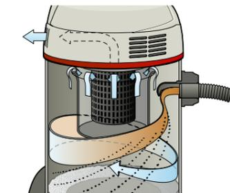
Due to the twist of the intake nozzle, the spray-fog is consequently diverted along the inner container wall. Additional filters are no longer necessary. The reliable floater system even reacts during heavy foam growth. Cooling air slots located on the side ensure the consistent separation of cooling and processed air.
