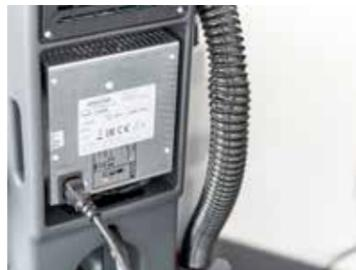
Internal charging station with battery runtime display.
