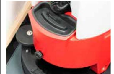
Rubberised guard roller allows for cleaning that is damage-free and close to floor edges.
